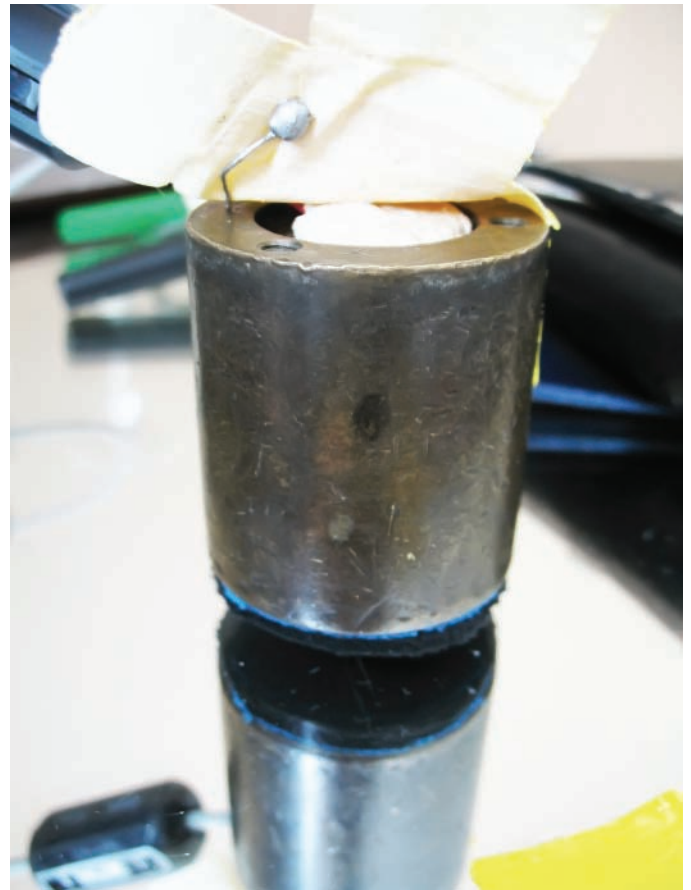
Fig. 2. Peppermint gum used successfully to repair broken solder joint Credit: China Blue.
