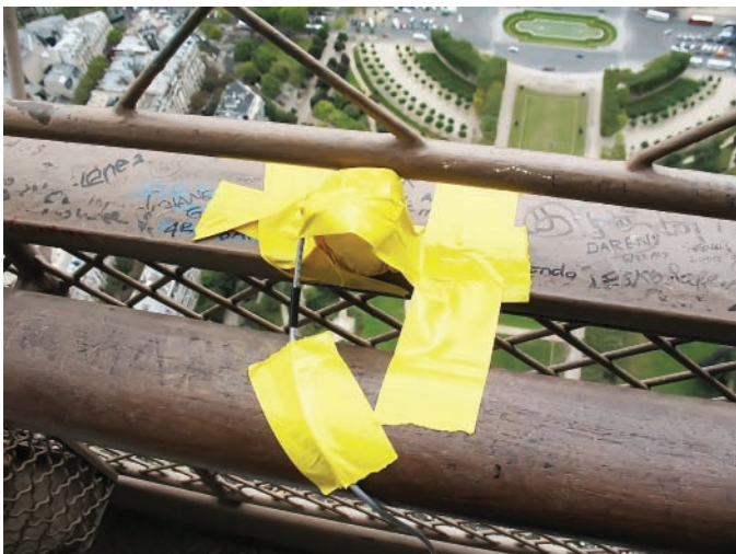
Fig. 7. Placement of the geophone on the railing with a view of the Champ de Mars below. Credit: Seth Horowitz.
